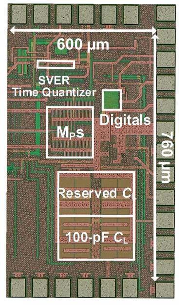
The smallest transient FOM and the best load regulation, while it used 0.5-V supply. And it had a small  $\Delta V_{OUT}$  by using SVER time quantizer
