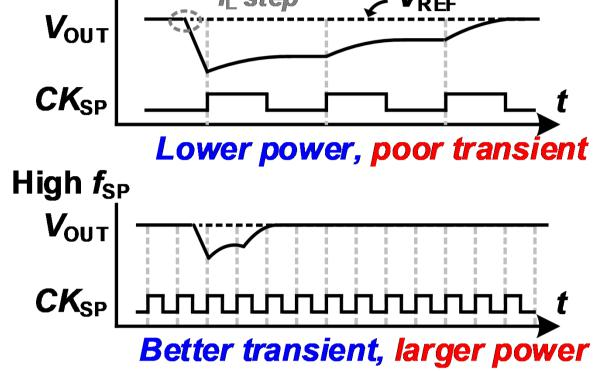
Digital LDO Using Multi-bit ADC [2]: Trade-off btw Power & Accuracy
